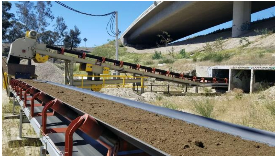
Figure 3. The conveyor belt system used to transport soil
